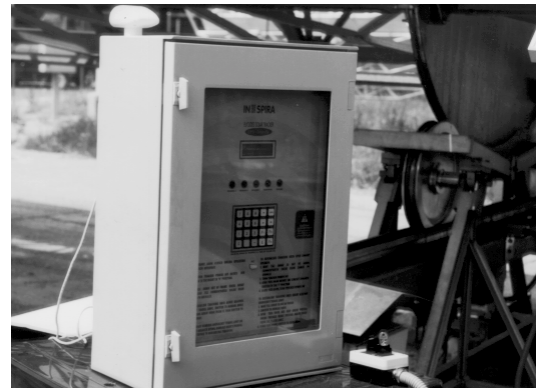
Figure 8: The tracking control box, (by INSPIRA).
